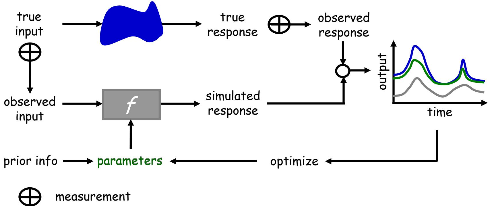
TUNING THE PARAMETERS SO THAT CLOSEST FIT TO THE OBSERVED SYSTEM RESPONSE IS OBTAINED
